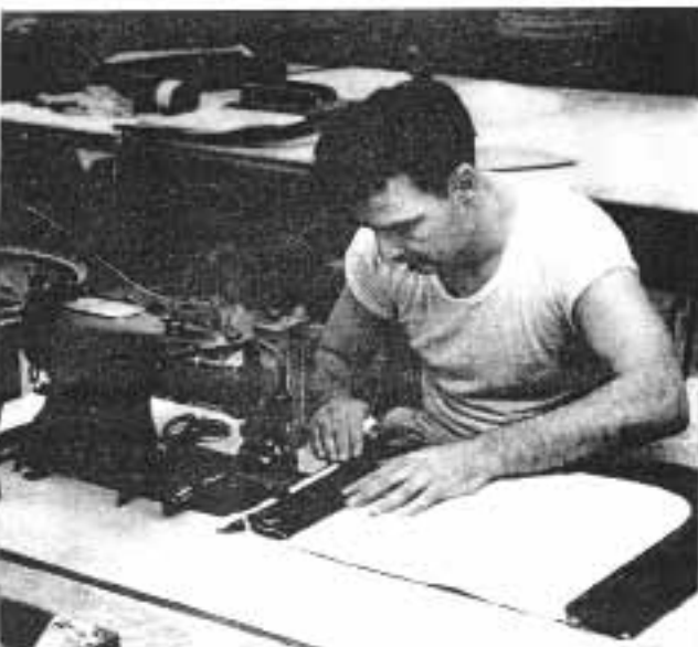
Some upholstery work for Owens cruisers is done in their own shop. Here a sewing machine operator works on the cover for a helmseat cushion.
