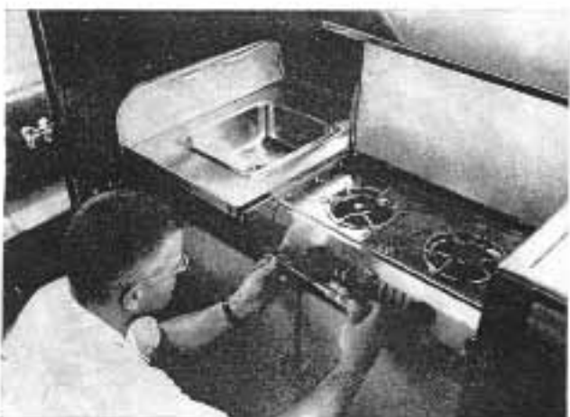
Galley tops have a hinged, stainless steel lid below which stove is placed. When stove is not in use lid folds down to make convenient work space.
